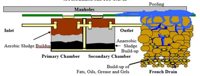
The Septic Tank is a concrete tank that receives waste from toilets, bathrooms, and kitchens. The tank has two chambers, the primary or solids chamber and the secondary or liquid chamber. There is a French drain or soakaway into which the liquid from the secondary chamber flows. The soakaway is the final treatment of the effluent and will vary in size depending on the size of the tank and amount of people the system is designed for.
